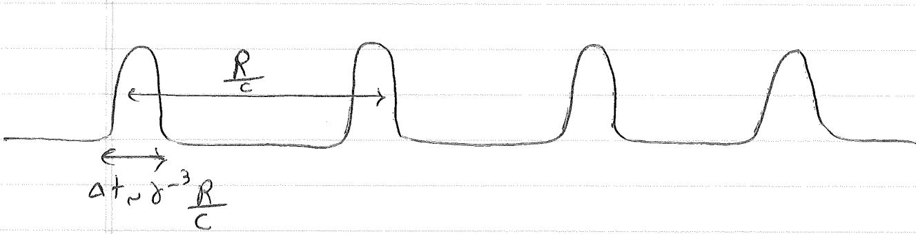
As a result, the spectrum of radiation covers all frequencies up to a maximum frequency  $\omega_{\max} \sim \gamma^3 \omega_0$ , where  $\omega_0 = \frac{2\pi R}{c}$  is the orbital frequency.
